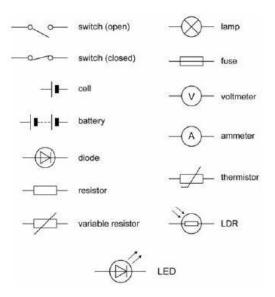
To measure current (I) - an ammeter is put in to the electrical circuit, unit is Amps (A).
