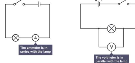
The **current** through a component depends on both the **resistance** of the component and the **potential difference** across the component.
